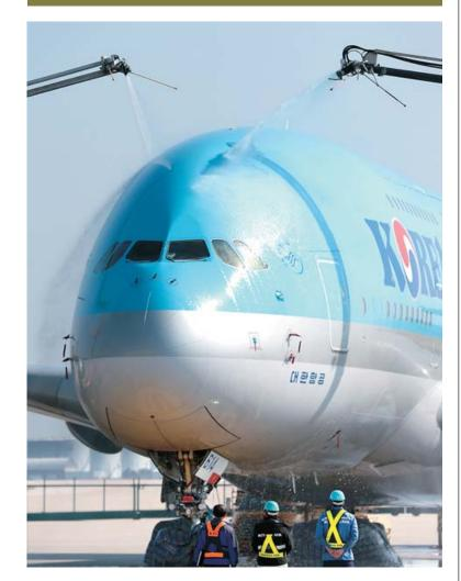
Spring cleaning A Korean Air A380 jumbo jet gets a wash at Incheon International Airport, Friday. It takes some 20 tons of water and 100 liters of cleaning fluid to wash the A380 plane, and around five hours to complete the task. The carrier regularly washes its planes to both make them clean and enhance their fuel economy. Yonhap
